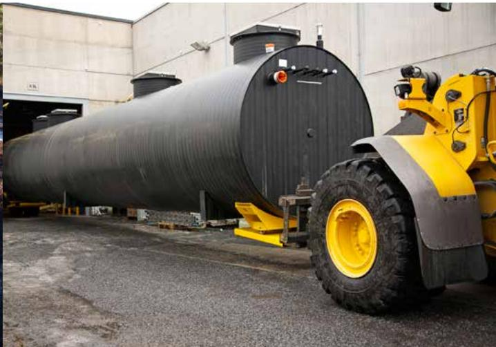
a WehoPuts 550 plant. The bedrock of Gotland mainly consists of limestone, which makes it difficult to build infiltration trenches. The municipality of Gotland does not grant individual properties the right to build wastewater treatment plants, at least four to six properties must be linked to the same plant.
