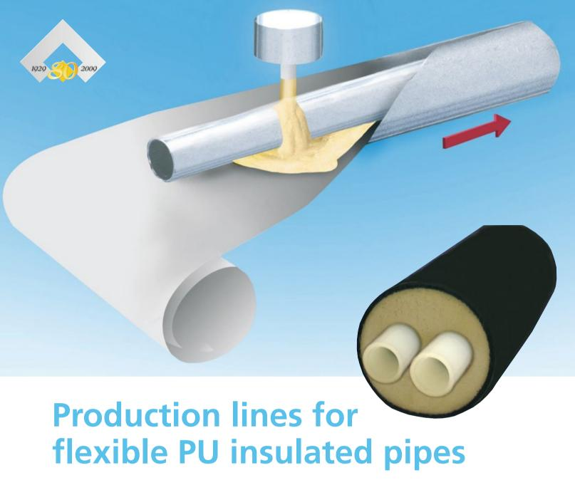
Flexible PU insulated pipes are manufactured on a continuous production line. The production machinery ilcludes decoilers, a film infeed unit, a foaming machine, laminator, extruder, haul-off and coilers. The pretreated plastic film provides a diffusion barrier, ensures excellent adhesion to the PU and welds to the external PE jacket pipe during the PE extrusion process.
